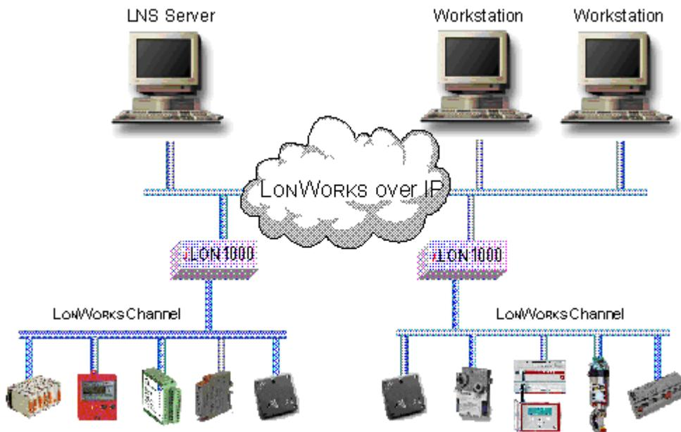
**Figure 12** Open LONWORKS Network with IP Backbone
