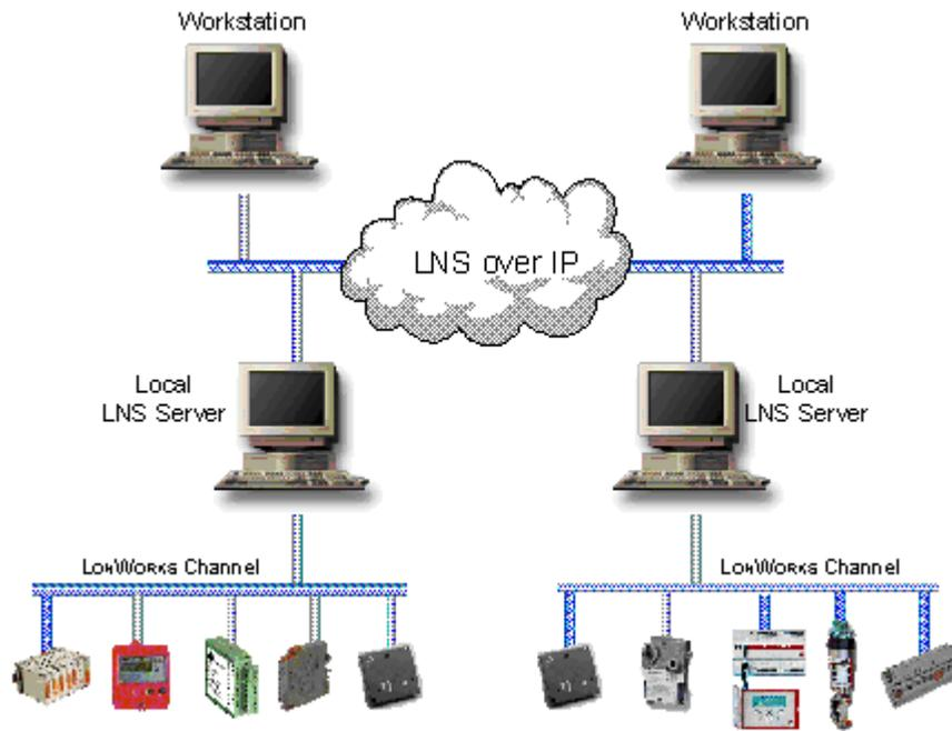
**Figure 13** Open LONWORKS Network with Local LNS Servers
